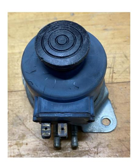
Switches to wiper motor and pump work, but there appears a small leak in the bellows
