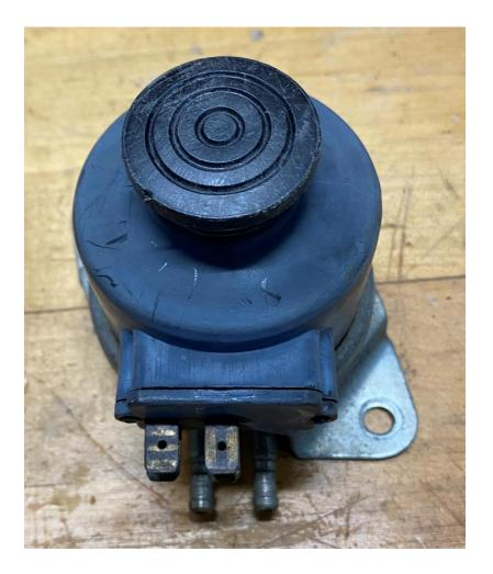
Switches to wiper motor and pump work, but there appears a small leak in the bellows
