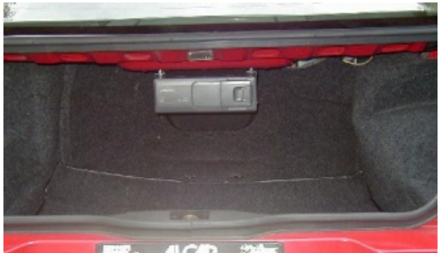
Here is the changer in place after the trunk interior carpets have been refitted
